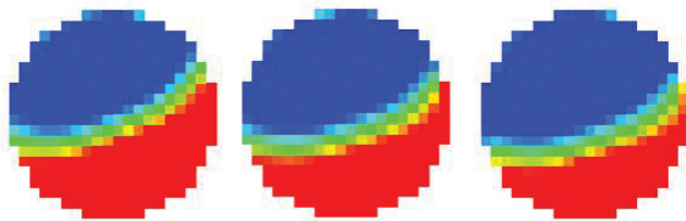
Figure 2: Cross-sectional conductivity tomographic images for 40, 50 and 60% oil.
