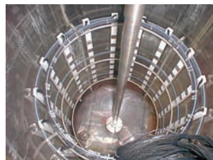
Figure 1: Multiple electrodes fitted to a stir tank
