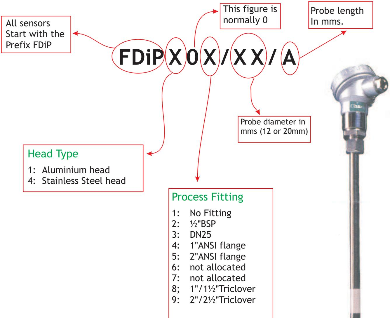
Using the key above, the sensor to the right is a FP101/12/500 - which is a 500mm long sensor with aluminium head and no fitting.
