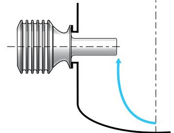
2.5 inch Sanitary or I-Line clamp and flow cell
