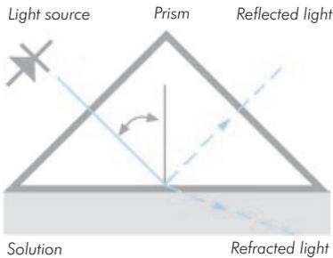
Depending on the angle, some rays are totally reflected. Some rays are only partially reflected, and most of the light is refracted into the process solution.
