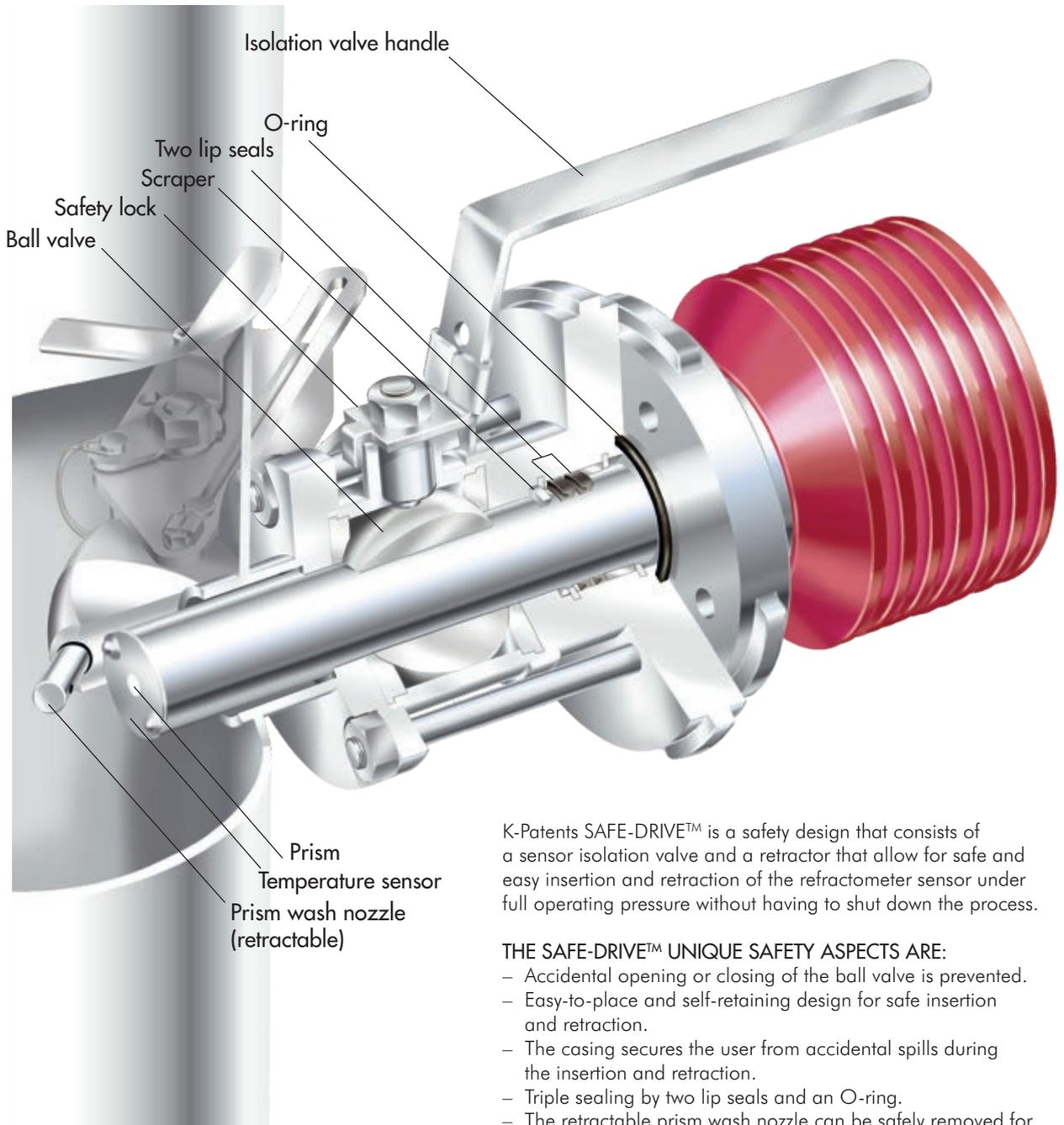
K-Patents SAFE-DRIVE™ is a safety design that consists of a sensor isolation valve and a retractor that allow for safe and easy insertion and retraction of the refractometer sensor under full operating pressure without having to shut down the process.
